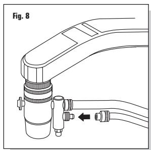
4. **Screw** the nuts onto the barbs and **hand tighten** (Fig. 9).
